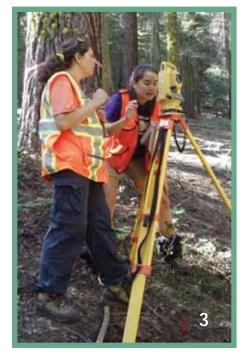
new student volunteers. They located the trees within each grid square using a basic station/off-set method using laser rangefinders, holding our final reprocessed coordinate values for each corner monument (remember the way we used to do topographic mapping – measuring down and out from the curb lines?). And yes, this year they too completed their task, and also did much rejoicing. In all, 35,000 trees were tagged!
